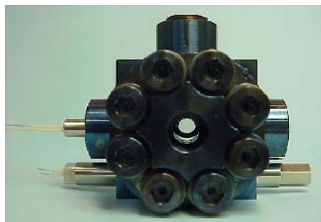
Fig. 1 Experimental cell for experiments on near critical pure water, in the High Temperature Insert inside the DECLIC CNES facility.
